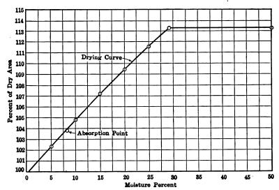
Fig. 62.—Relation between the moisture content and the cross section of small, clear specimens of western larch.
